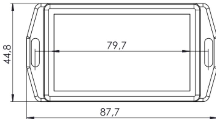
To easily mount the sensor, copy this mounting template (scale 1:1).
