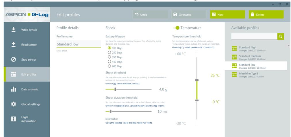
**Please note:** the data rate is the higher, the shorter you define the lifespan of the battery. A high data rate is useful especially for the recording of short shocks.
