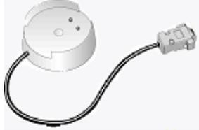
Place the logger into the **Interface**, making sure that the two metallic contacts on the bottom of the logger are aligned with the contact pins on the **Interface** and that the logger is firmly seated. The software defaults to "auto-detect" mode, which will check all the installed serial communications ports (COM) on your computer for a logger, ChartReader, or other known Escort products.
