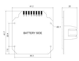
The PCB edge mates with a 0.1" IDC female edge connector, such as RS Part No. 471-317.
