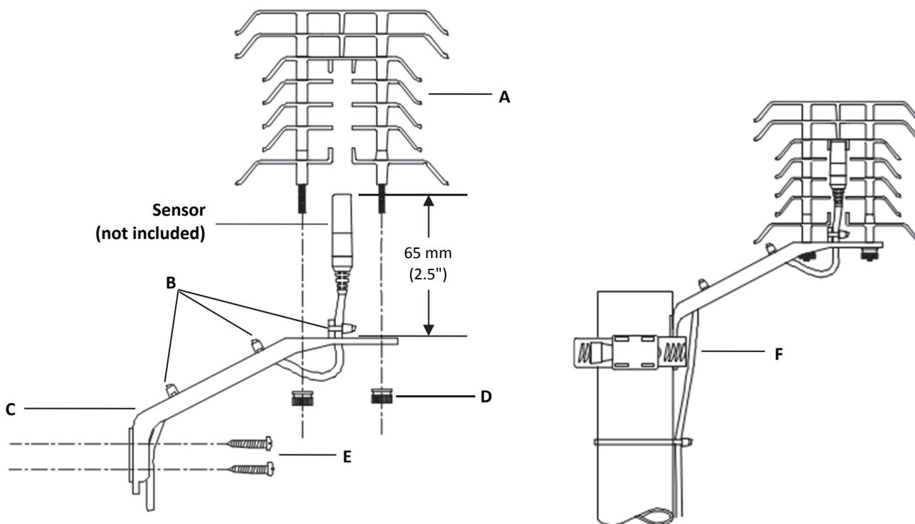
**Note:** This shield does not protect sensors from light reflected from below the shield at some angles. Avoid deploying this shield next to reflective surfaces if possible.
