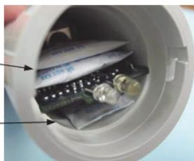
7. Re-install end cap. Make sure the O-ring on the end cap is still in place. It should not be pinched, twisted, or trapping dirt or lint, which could interfere with the end cap. Line up the two small bumps on the end cap with the two notches at the end of the case and then push end cap in and lock into place by turning clockwise just slightly until bumps prevent further rotation.
