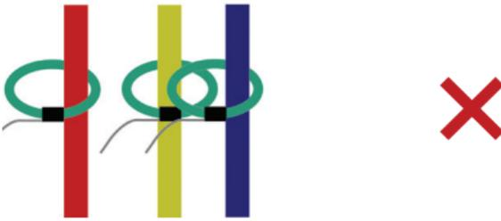
The coil around the blue conductor is too close to the yellow conductor. Ensure that coils are not positioned too closely to neighbouring conductors.
