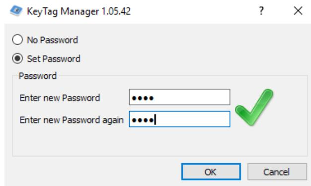
The new password is now set. The logger can be configured. This password will be written into the logger. When this logger with a password is reconnected, all the configuration controls are disabled including the configure button. Until the right password is entered.
