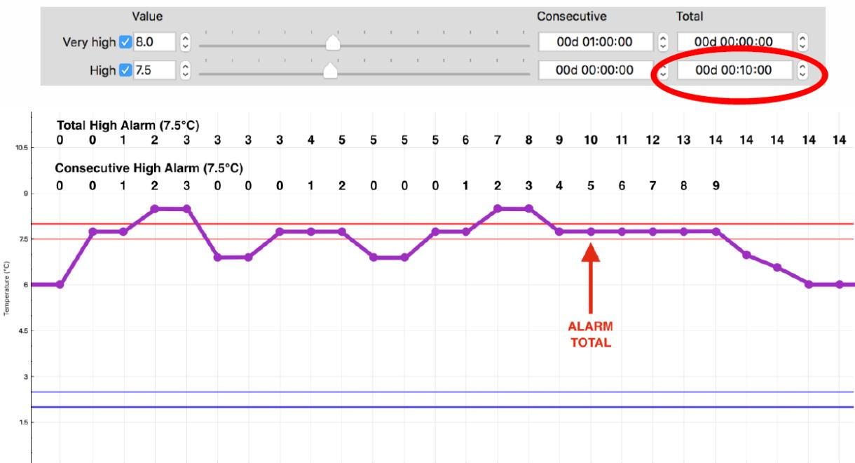
Example: High alarm threshold set to 7.5°C with a consecutive delay of 6 minutes and a total delay of 12 minutes. The sampling rate is 1 minute. In this scenario we have both, the consecutive, and the total delay set respectively to 6 and 12 minutes. In that example, the alarm is triggered when the consecutive delay reaches 6 minutes.
