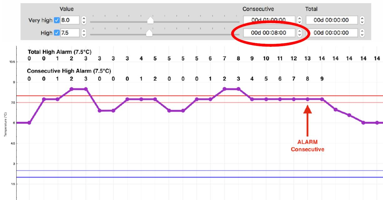
Example: High alarm threshold set to 7.5°C with a total delay of 10 minutes and no consecutive delay. The sampling rate is 1 minute. The alarm is triggered when the total delay reaches 10 minutes. As we can see in this example, the counter stopped counting when the temperature goes back below 7.5°C and continues when above 7.5°C.
