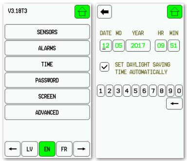
(4) Tap , then choose Sensors menu and tap the Setup button. Set up a sensor by following the instructions on the screen. After successfully setting up a sensor, the sensor ID and the name of the sensor will appear on the left side of the screen. Sensors are given name "SENS <number>" automatically. Tap the name of the sensor to give it a new name with length up to 8 symbols. In order to remove a sensor just press the sign next to it.
