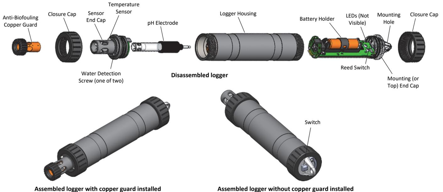
**Anti-Biofouling Copper Guard:** Use this guard to protect the pH electrode when deploying the logger in water prone to biofouling (see *Deploying and Mounting the Logger*).
