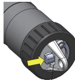
Push switch into the gap beneath the mounting lanyard to start or stop logging or to wake up the logger
