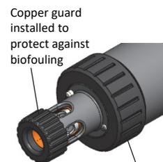
Copper guard installed to protect against biofouling
