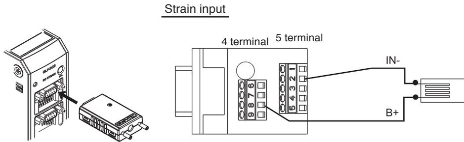
How to assemble the DSUB-Screw terminals conversion connector (Optional B-561)
