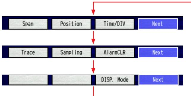
Time/DIV : Changes the time scale. (For details, see "(14) Waveform setting (Simple Waveform Setting)" on page 3-112).
