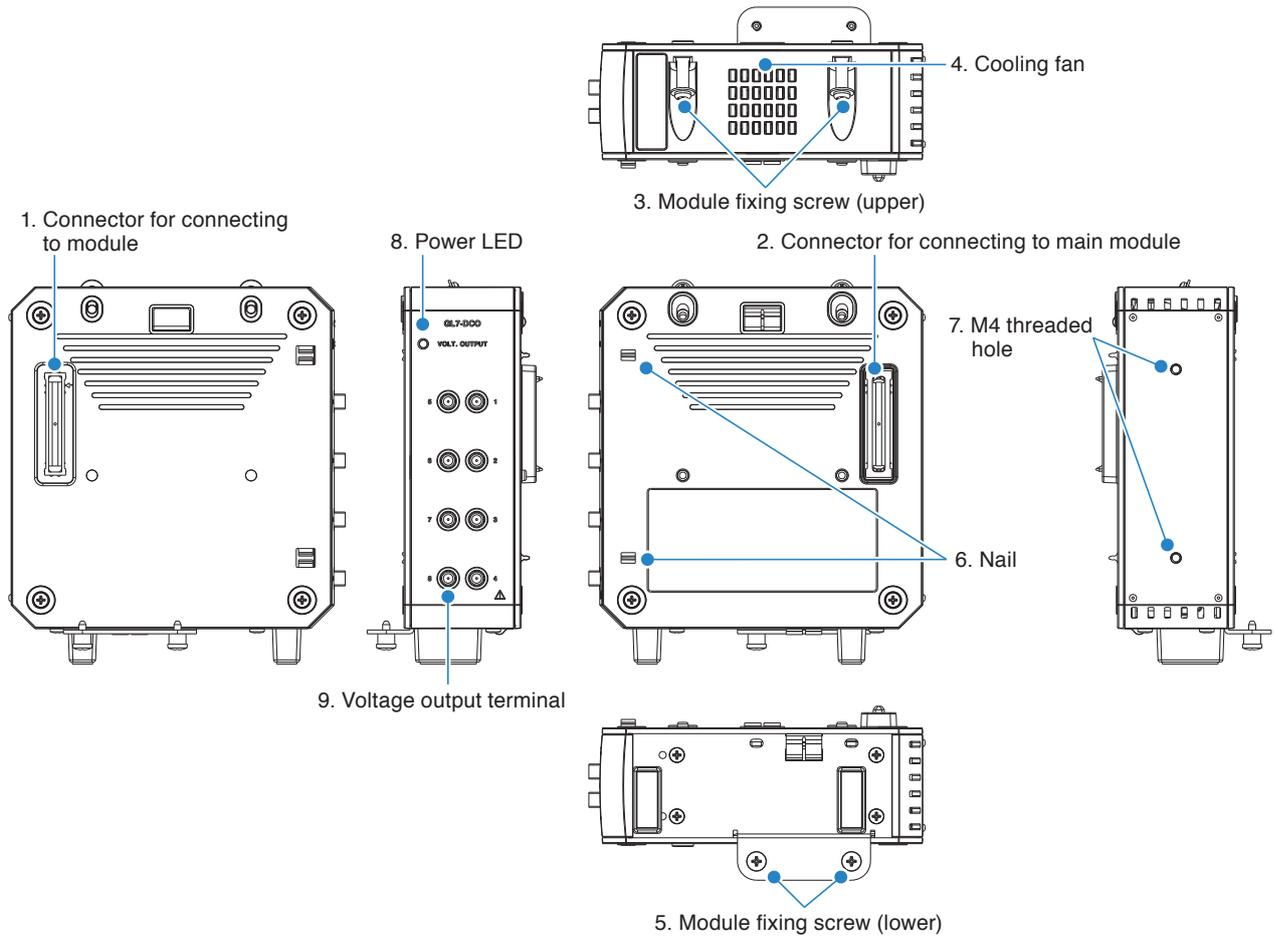
1. Connector for connecting to module .....Connector for connecting to the various modules.
