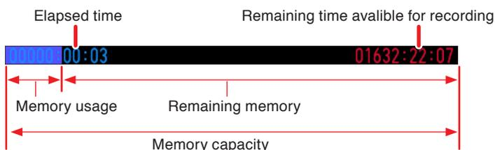
For example, for a 2GB SD card, where approx. 768MB is being used, the memory capacity is 2GB, used memory is approx. 768MB, and the remaining memory is approx. 1.25GB. As recording time elapses, the memory used increases and the remaining memory decreases.
