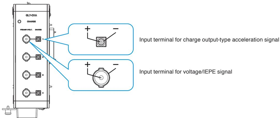
+ ..... High-voltage terminal (Terminal for inputting the high-voltage side of the input signal)
