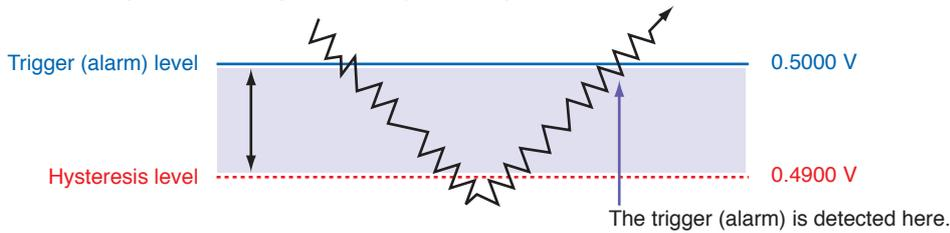
\* For Rising mode, when the signal level drops below the hysteresis level at a time, and then becomes greater than or equal to trigger (alarm) level, the trigger (alarm) is detected.
