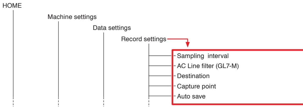
Pressing the "Capture" icon moves the user to a settings screen with set items such as "Sample Interval" (the red framed part on the chart above).
