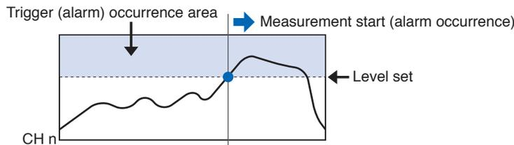
Low: Condition where a trigger/alarm occurs when the input signal exceeds a set level.
