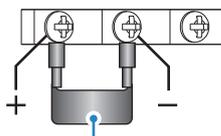
Example: In the case of 4-20 mA, apply 250Ω (±0.1%) and measure in the 1-5 V range.
