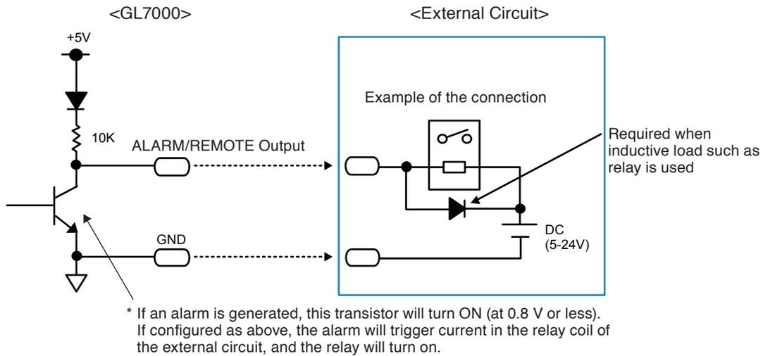
**GL input and output cabling**
