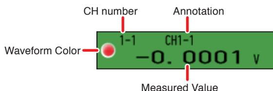
Waveform Color : The waveform color currently set. (For details, see "(11) Input settings" on page 3-78.)
