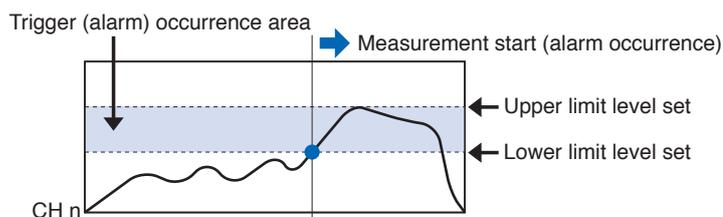
Win out: Condition where a trigger/alarm occurs when for any channel, the upper and lower limit value is set, and an output signal between those levels is output (when a signal is output)
