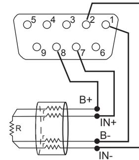
When measuring the resistance, as shown in Figure above, wire using the following 4-wire, or short between (1) and (2), and (7) and (8).
