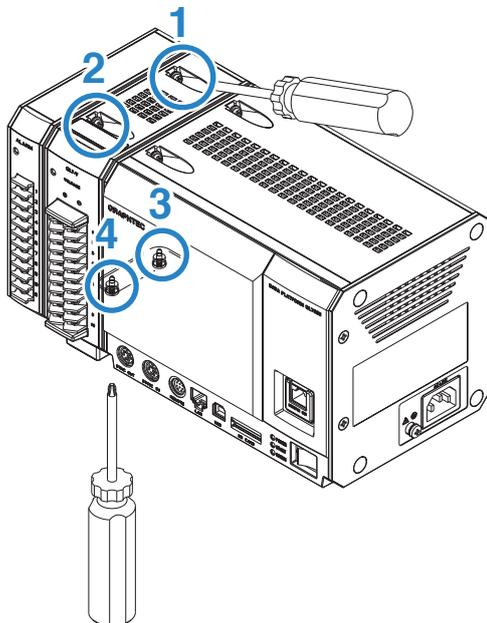
**When installing multiple modules**
