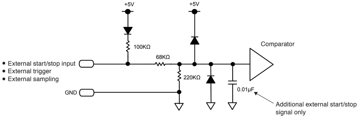
**REMOTE signal input circuit**
