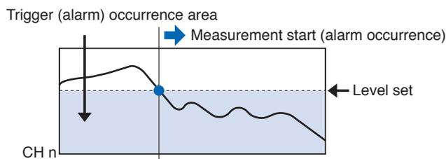
Win in: Condition where a trigger/alarm occurs when for any channel, the upper and lower limit value is set, and an input signal between those levels is input (when a signal is input).
