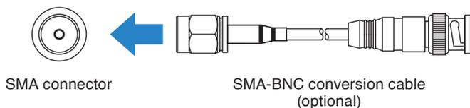
If you do not use the cable sold separately, always connect with the cable that conforms to SMA connector specifications.
