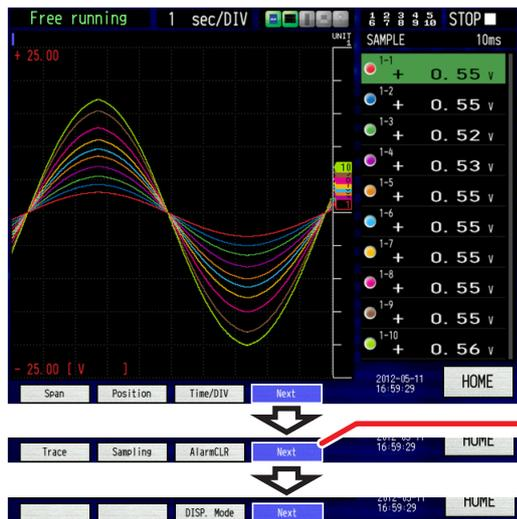
Each time you touch the "Next", the function of the Function button is changed. The Function button allows you to modify the time scale, to process the waveform, to set the sampling, to clear the alarm, and to change the display mode.
