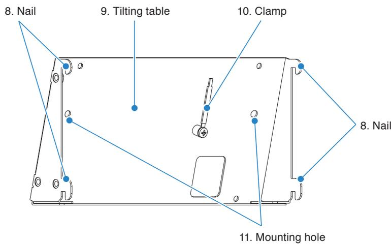
8. Nail .....Nails for fixing to the main module (4 places).
