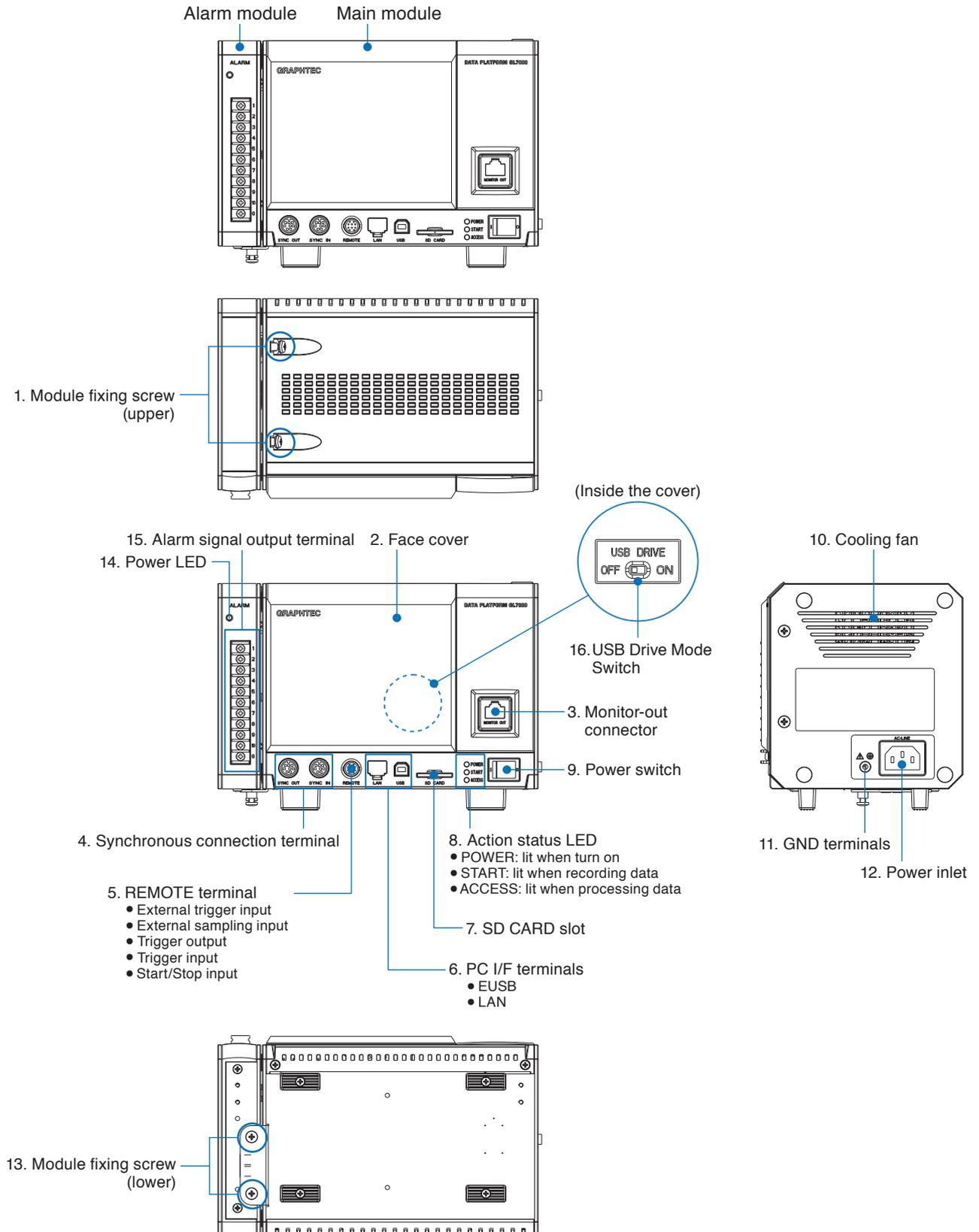
1. Module fixing screw (upper) ..... Fixation screw for the adjoining module.
