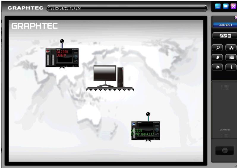
When the GL7000 and the PC are connected correctly, and when the power to the GL7000 is turned on, the GL7000 should be automatically recognized and the GL7000 equipment icon should be displayed. If the equipment icon isn't displayed correctly, see "6.5 GL7000 Interface Settings."
