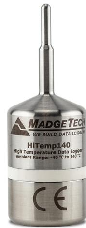
The HiTemp140 is a rugged, high precision, temperature data logger that is built for use in harsh environments. This stainless steel device is submersible and can withstand temperatures up to 140 °C (284 °F). With the HiTemp140's standard calibration, an accuracy of  $\pm 0.1$  °C ( $\pm 0.18$  °F) can be achieved over a wide temperature range.
