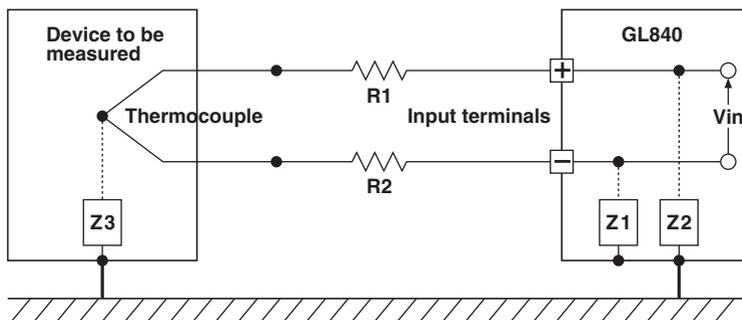
Ex 2 : Connect GL840's GND to measurement object's GND.
