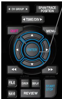
(3) Push the [ENTER] key according to the "Level Settings" . The "Trigger Level Settings" screen is displayed. Move the cursor to the "Mode" parameter for the CH1, and then select "H".
