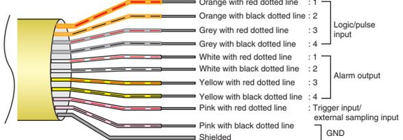
\* The B-513 input/output cable for GL (sold separately) is required for connecting input/output signals. (For logic/pulse input, alarm output, trigger input and external sampling pulse input)
