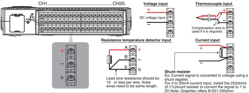
CAUTION: Connect wires to the specified channel, the channel number is shown on top of the terminal block.
