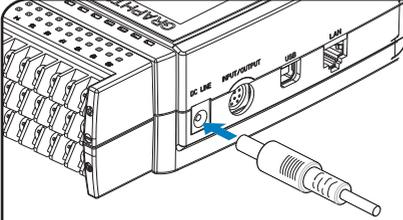
Connect the DC output of the AC adapter to the connector marked as "DC LINE" on the GL840.
