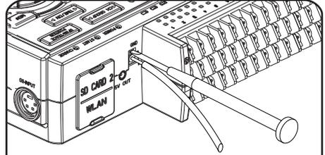
Use a flathead screwdriver to push the button above the GND terminal while connecting the ground cable to the GL840. Connect the other end of the cable to ground.
