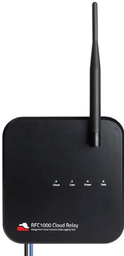
The RFC1000 Cloud Relay allows data from MadgeTech wireless loggers to be sent directly to a MadgeTech Cloud Services account, eliminating the need for a central PC and MadgeTech 4 Software. With the RFC1000 Cloud Relay, real-time data can easily be transmitted to the MadgeTech Cloud, where it can be viewed from any Internet enabled device.
