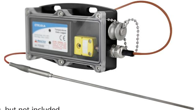
Setup is fast and easy. The 1/4" NPT coupler is attached to the exhaust pipe; the use of a compression fitting allows for the thermocouple to be placed directly in the exhaust stream, providing for highly accurate profiling. The data logger, which is contained within the weatherproof enclosure, is then mounted to the vehicle.
