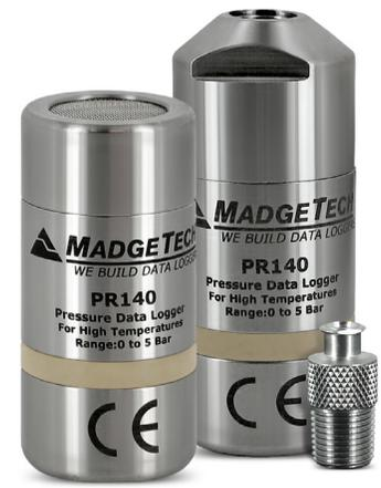
The PR140 is a pressure data logger designed for use in autoclave validation and mapping. This rugged device can withstand temperatures up to 140 °C and is completely submersible (IP68).
