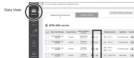
The signal strength between Base Unit and Remote Unit can be checked by color and number of antennas.
