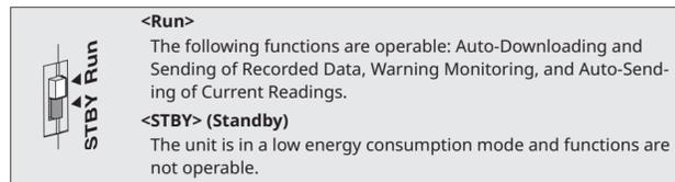
\* After the switch is set to <Run>, the unit will start operating in 2 minutes or less (depending on the number of registered Remote Units and Repeaters).
