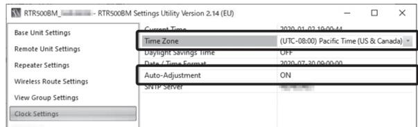
\* Auto-Adjustment is a function to automatically adjust the date and time of the Base Unit using the SNTP server. Clock adjustment is made when the Operation Switch is turned to the <Run> position and once a day.
