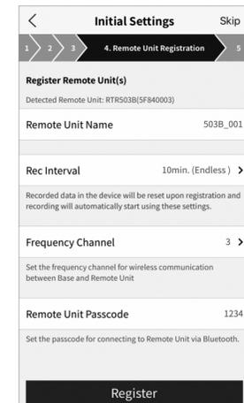
\* When more than one Base Unit is registered, make sure to select channels that are far apart in order to prevent interference of wireless communication between the Base Units.
