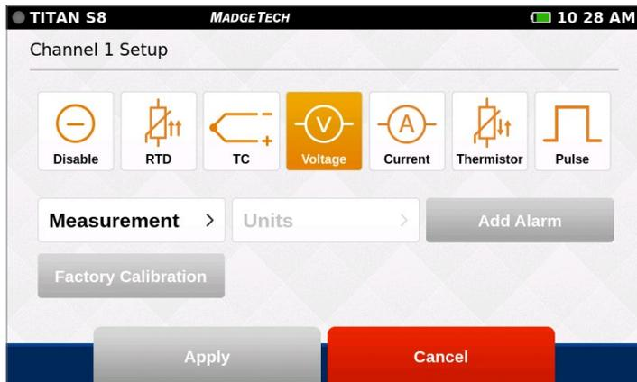
**Factory Calibration:** Indicates the device is currently in the factory calibrated state.
