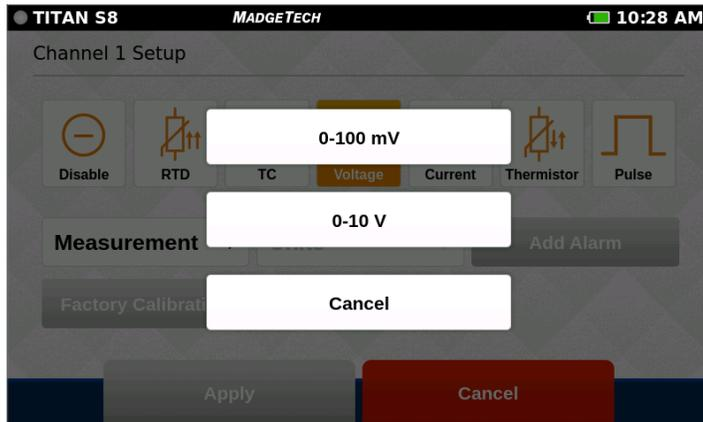
Select the **Measurement** button to display a pop-up screen of relevant measurement types to choose from.
