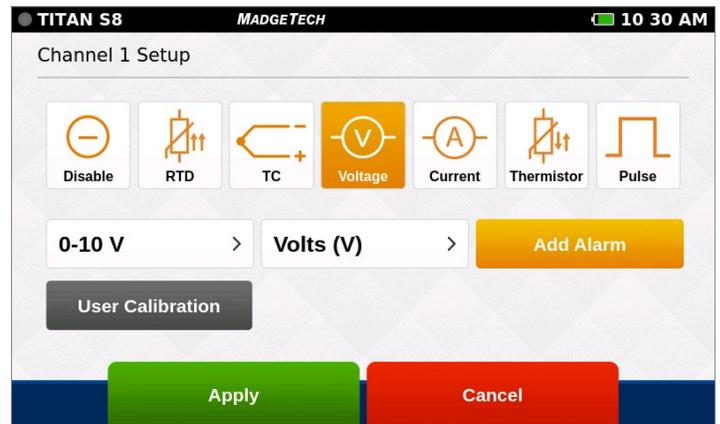
**User Calibration:** Indicates the calibration settings have been modified by the user.
