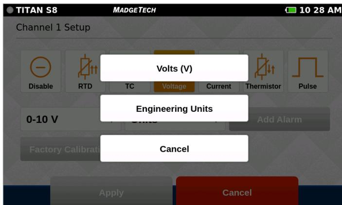
**Engineering Units:** This will be an option to set up if the user selects the Voltage, Current, Frequency or Pulse sensor (see details below and on [page 9-10](#)).
