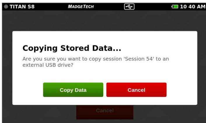
**Note:** Data can be saved to external memory as .csv and/or .mtb file format (user selectable in System/File Format). Saving as .mtb file format will allow data to be imported into MadgeTech 4 Data Logger Software (version 4.2.13.0 or greater).
