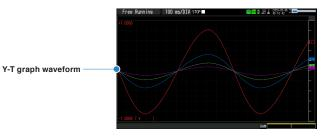
With this display format, you can display the time axis of Y-T graph waveform can be views wider by hiding the digital display.
