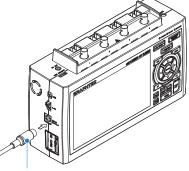
Input/output cable for GL (B-513: Option)
