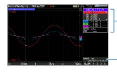
Displays the voltage at a point indicated by Cursor A or B or the selected cursor.
