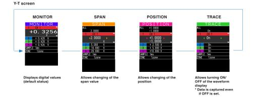
Use [CH SELECT] key or the  $\blacktriangle \blacktriangledown$  keys to move on the CH.
