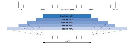
When the Vernier is set to 100%, it magnifies equally along the axis. Therefore the waveform display reflects the Vernier setting magnification.
