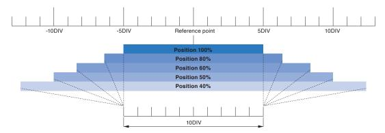
When the VERNIER is set to 100%, it becomes an equal magnification. Therefore the waveform display is shrunk by the VERNIER setting magnification.
