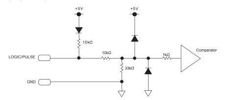
• Trigger input/external sampling input
