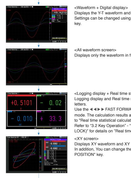
Displays the Y-T waveform and the Digital display. Settings can be changed using the [SPAN/TRACE/POSITION]
