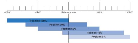
As shown in the above figure, the display range moves in parallel with 10DIV area with the XY position setting.
