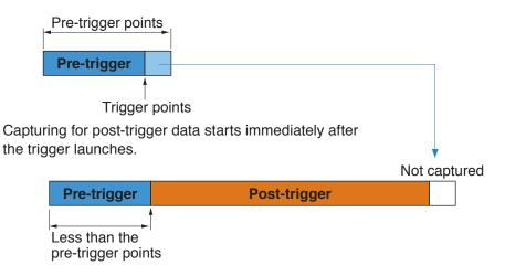
The total data after capturing is less due to the uncaptured pre-trigger point.
