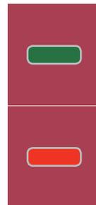
**Green LED blinks:** 10 seconds to indicate logging and 15 seconds to indicate delay start mode.
