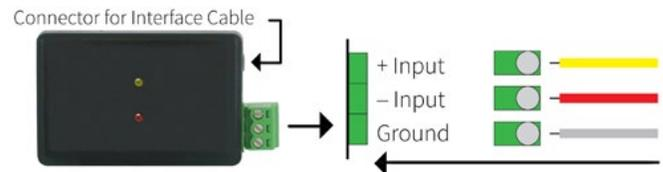
The TC101A-ST and TC101A-TB have the ability to shield the thermocouple with the ground connection. When using a 2-wire thermocouple, leave the ground input unconnected.
