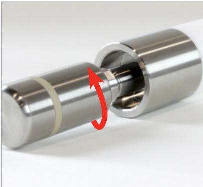
3. Unscrew the HiTemp140-M12 data logger, from the lid of the thermal barrier.
