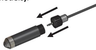
**Important:** Make sure the O-rings on the cable jack end and the cable and sensor mating housing surfaces are clear of any debris. Any contamination of these surfaces can cause leaks that may lead to sensor failure.
