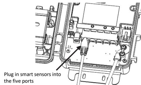
Plug in smart sensors into the five ports
