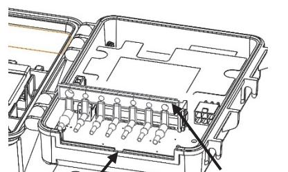
Notch where the key on the bottom of the cable channel is installed
