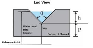
The HOBOlink water flow calculations for a v-notch weir assume the following:
