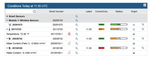
• Click Devices, then Map, and hover over a mote to see the connectivity level. This also shows the signal level, which indicates how strong the wireless signal is between motes (this is also available on the mote LCD). Signal strength correlates with network connectivity: the stronger the signal, the better the network connection.
