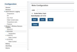
4. If the mote you are deleting is currently active on the network (i.e. powered up and transmitting data), the station will need to connect to HOBOlink to complete the removal process. Otherwise, the mote will not officially leave the network and can attempt to automatically rejoin the network in the future. To connect to HOBOlink, press the Connect button on the station. Once the station is connected, a command is sent to the station and the mote permanently leaves the network.
