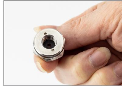
1. Ensure the sealing ferrule is seated inside the receptacle. Use the black rubber ferrule for 0.080 - 0.100 inch diameter probes or the red rubber ferrule for 0.100 - 0.125 inch diameter probes.
