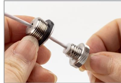
3. Insert data logger probe tip through the receptacle.
