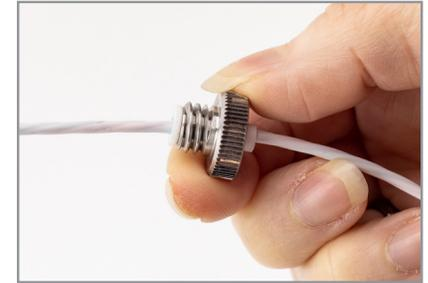
2. Thread the data logger probe through the thumb screw as shown.
