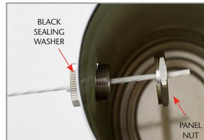
5. Place the black sealing washer over the probe tip and insert through the 9/16 inch diameter hole of the container from the outside. Place the panel nut over the end of the probe tip as shown from the inside of the container and thread the two pieces together.
