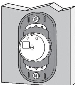
Use two #8 screws (not included) to mount the logger in the boot to a flat surface. Do not overtighten the screws.
