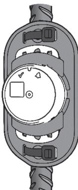
Use two of the included zip ties to mount the logger in the boot to a small pipe as shown
