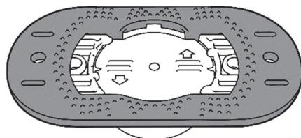
Insert the other logger mounting tab into the boot, making sure the logger is securely seated in the boot as shown
