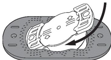
Holding both the boot and the logger upside down, insert the logger mounting tab into the boot as shown
