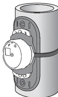
Use one of the included zip ties to mount the logger in the boot to a large pipe as shown
