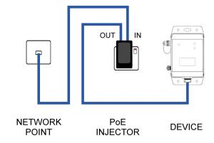
Once connected, turn the PoE injector on.
