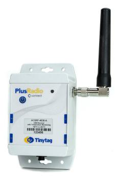
Tinytag Plus Radio data loggers are a range of wireless data logging products designed for outdoor and industrial use. The receiver is used as part of a Tinytag Connect system that forms a robust data network that allows a user to see the conditions within an application from their own desk, across a LAN or the Internet.
