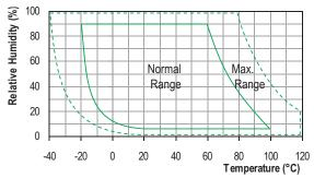
Long term exposure to humidity levels outside of the 'normal' range may temporarily offset RH measurements (±3%RH after 60 hours). Once returned to less extreme conditions the device will slowly return towards calibration
