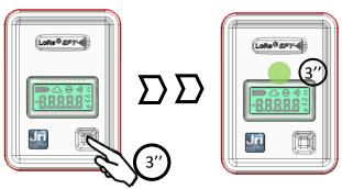
Once activated, the LoRa® SPY measures and transmits its measurements to My Sirius, at the frequency defined in MySirius, then flashes regularly as a function of its status.
