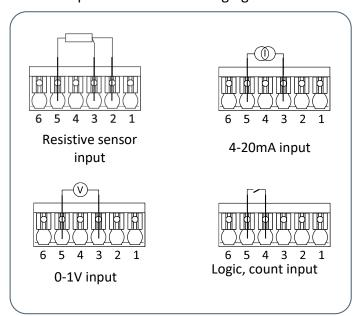
/!\ Connect only sensors which are compatible with the technical characteristics of the devices Sensor default detection is not possible in 0-20mA and 0-1V.
