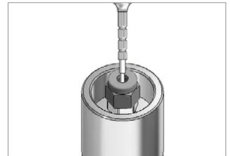
5. Feed the data logger probe through the Compression Fitting until the base of the probe is tightly against the Dome Nut.
