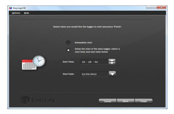
To delay the start of the data logger to a preset time and date, select that option and select the Start Time (hh:mm:ss format) and Start Date (dd/mm/yyyy format) at which you want to start logging, and click on the Finish button.
