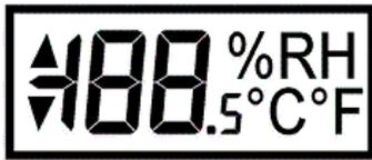
The LCD on the data logger provides information on the logging status of the unit at the touch of a button. The table below shows the various displays possible.
