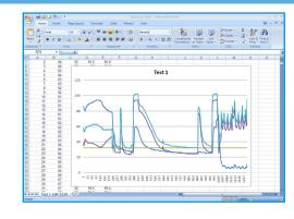
Retrieve data by connecting the logger to a computer through USB or by removing the SD memory card and inserting it into a computer.
