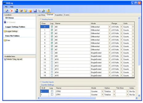
DAQLog software is included to configure the device, set up channels and logging parameters, and to retrieve data
