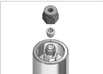
4. Insert the Compression Ferrule into the Fitting Body and hold it in place loosely with the Dome Nut.
