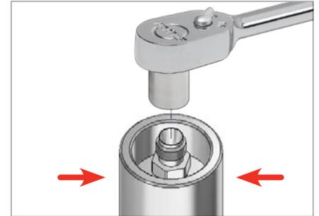
3. Holding the smooth metal end of the stopper, use a 7/16" wrench or socket to tighten the body into the stopper.
