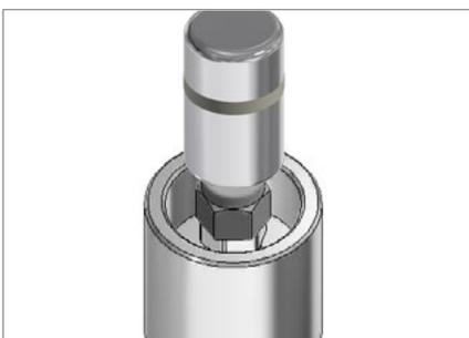
6. Tighten the Dome Nut to secure the data logger in place (finger-tight).
