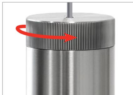
7. Insert the data logger and stopper assembly back into the thermal barrier and screw the endcap of the thermal barrier until the O-Ring is no longer visible.
