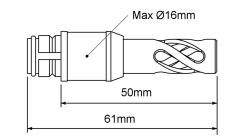
IP Rating IP20 Operational Range\* -25 °C to +85 °C Dimensions Probe Length (excluding cable) 61mm / 2.4" Maximum Diameter 16mm / 0.63" Cable Length 1.5m / 59.055' Weight 10g / 0.35oz
