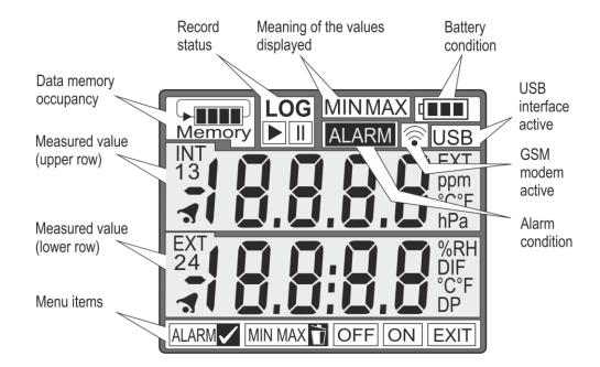
**Data memory occupancy** - this display section offers information about the current condition of the free space existing in the data memory. The blinking of the *Memory* symbol indicates that the preset memory occupancy limit has been exceeded. This limit can be set up in the device's configuration. Several actions can be assigned to it (optical and acoustic signalling, sending SMS messages).
