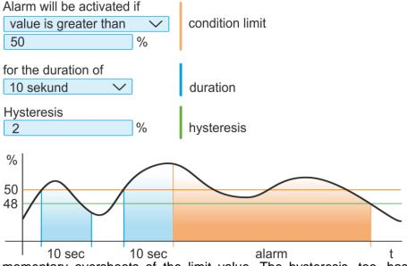
momentary overshoots of the limit value. The hysteresis, too, has a similar significance (*Alarm hysteresis*). It prevents the alarm from oscillating in the case that the measurement value varies around the alarm limit value. It is not recommended to set it equal zero.
