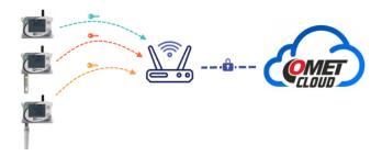
COMET WiFi sensors send data into COMET Cloud at selected interval via common 2.4 GHz WiFi infrastructure. WiFi sensors are equipped by own non-volatile memory for samples which cannot be sent in case of WiFi or ISP connectivity outage.
