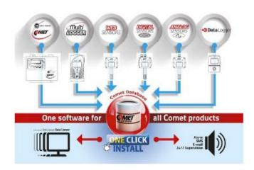
For customers which cannot use 3rd party Cloud service from the security reasons or users which want to execute data acquisition system at own server infrastructure is here COMET Database solution. COMET Database is a solution using Microsoft SQL database server as data storage and Viewer software installed at client stations.
