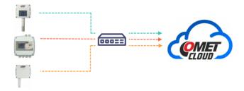
COMET Web sensors send data into COMET Cloud via Ethernet infrastructure. Measured values are sent via SOAP protocol transported by HTTP transfers.
