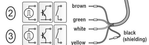
! The binary inputs are not galvanically separated (green, yellow and black wire are inside the device connected to one point) !
