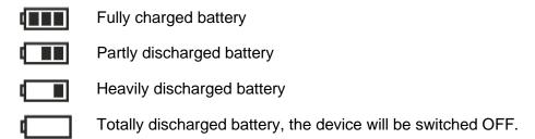
Battery conditions with a charger connected to the battery:
