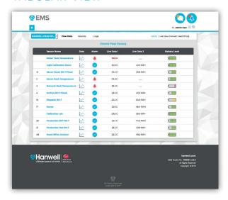
**Tabular View** provides list of sensors with clear indication of alarm, battery status and live data
