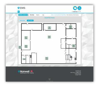
**Plan View** provides visual indication of sensor location within a facility. Sensor icons show real-time data and alarms and interaction by double clicking icon.
