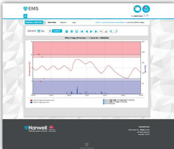
**Graphical View** provides line graphs with optional door position indicator, alarm level indication. Data overlays, zoom plus many more features.
