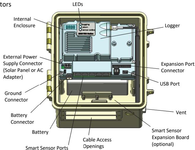
**Important:** Always plug in the battery first, before plugging in any solar panel or power supply connector. When disconnecting power, always unplug any solar panel or power supply connector first, then unplug the battery.
