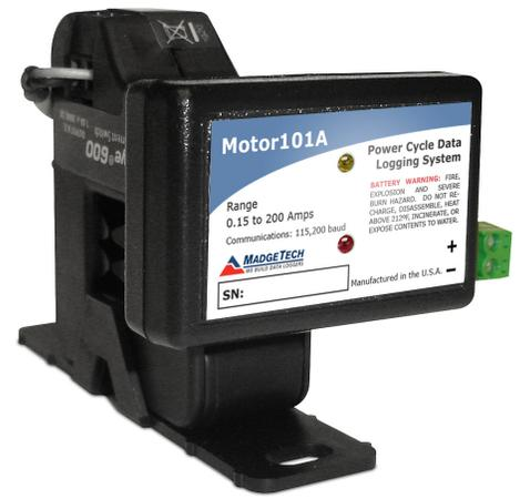
The Motor101A measures and records on and off status changes for motors or other equipment drawing up to 200 Amps. The state change occurs when the current switch exceeds the 150 mA set point. This allows for most basic equipment to be monitored.
