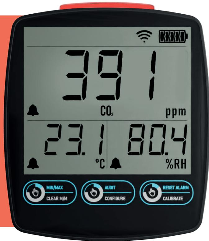
The EL-IOT-CO2 continuously monitors air quality and comfort levels, including CO<sub>2</sub>, a key indicator of adequate ventilation. It automatically uploads data to the EasyLog Cloud, allowing your complete set of data measurements to be viewed, analysed and downloaded from any internet-enabled device.
