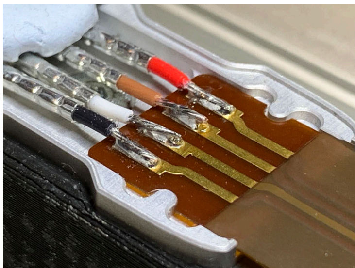
Figure 7.2.2 FHF04 sensor foil with soldered wires.
