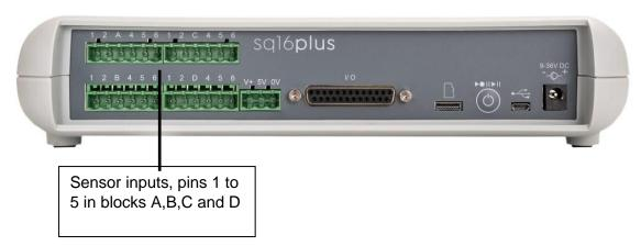
There are 5 different types of channels that may be measured and recorded by the sq16, and sq16plus loggers, these are:
