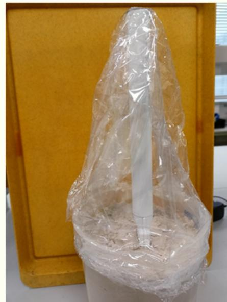
Figure 2: Food foil cover preventing water evaporation
