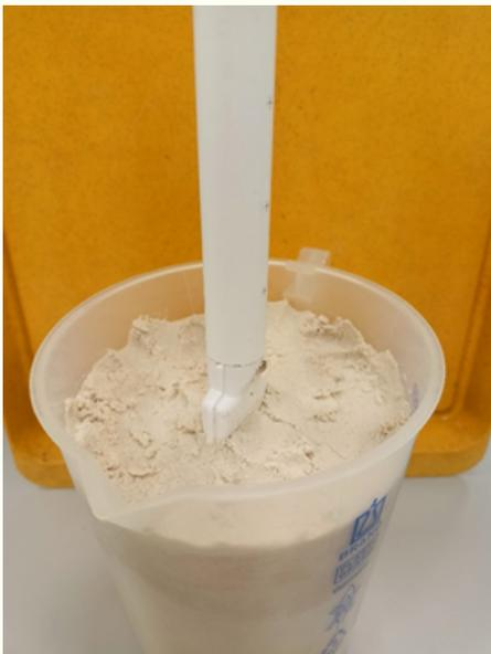
Figure 1: Placement of datalogger in sandy soil
