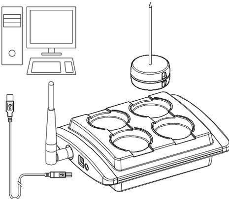
For programming the data loggers and for reading the recorded data, they are placed in the interface.
