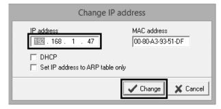
• gateway may not be entered if you want to use the device only in local network. If you set the same IP address which is already used, the device will not work
