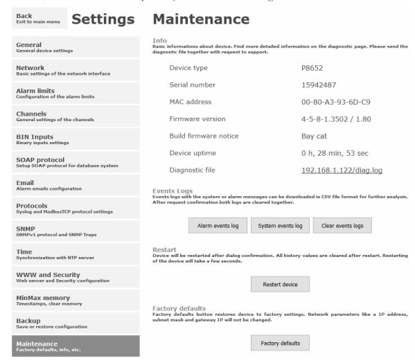
Network parameters are changed when factory default button is pressed during device power on (in more detail – see Chapter 5).
